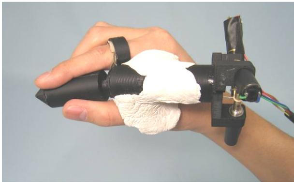
Fig. 5. Prototype device grasped by hand
