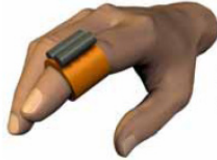
Fig. 2: Schematic illustration of the haptic interface for middle phalanx (The device will put on every finger).
