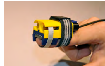
Figure 1. The finger-worn haptic display using dual motors
