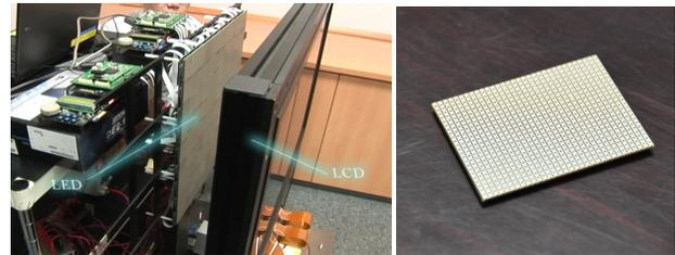
**Figure 3.** (Left) Construction of the 3D display using a LED panel as light source and a LCD panel as dynamic parallax barrier. (Right) Our developed high-density LED module
