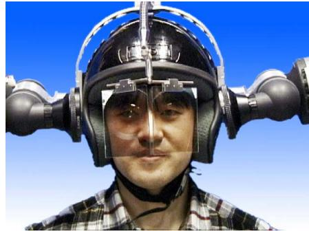
Fig. 12 Head Mounted Projector (HMP) with RPT.
