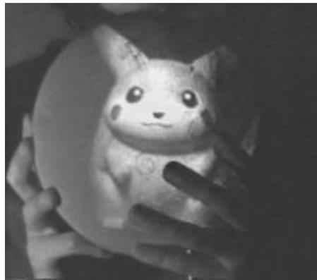
Fig.13 Projected image on a spherical retro-reflective screen.
