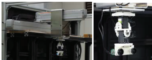
Figure 4: Completed robot camera with the 2 DoF linear servos above the 3 DoF robot head with the stereo camera.
