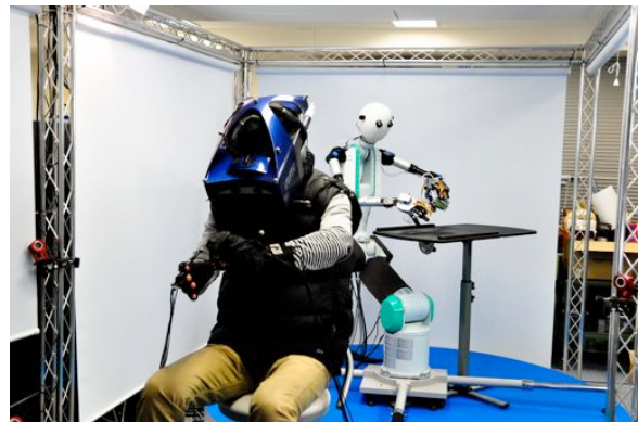
Fig. 1 TELESAR V in a glass ball pouring Tele-operation
