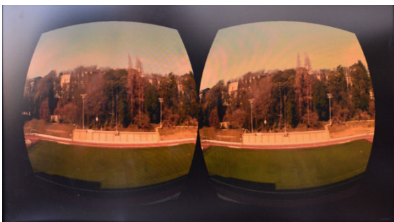
Fig.7 Rendered Video displayed in HMD(Oculus Rift)
