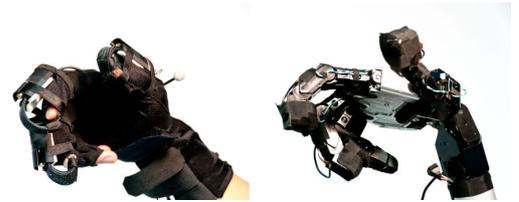
Figure 6: Master Glove vs. Slave Hand
