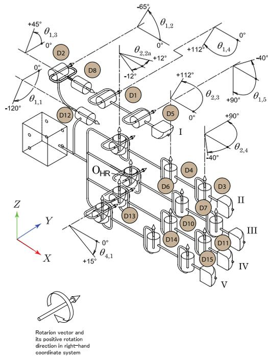
Figure 7: 15 DOF Anthropomorphic Robot Hand Coordinate Frame Assignment
