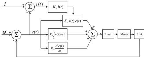
Figure 8: Control Logic Block Diagram for 15 DOF Hand
