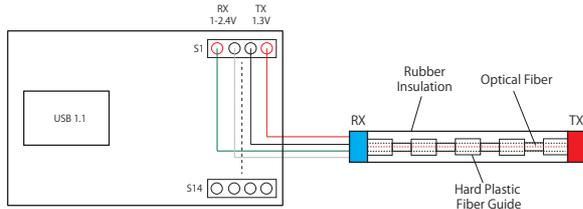
Figure 5: Optical Bend Sensor Internal Structure
