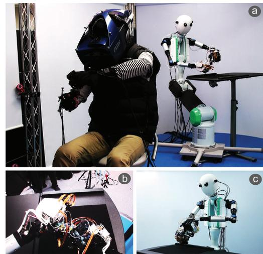
Figure 1: (a) Master-Slave Configuration, (b) Slave Hand as seen from the HMD, (c) Slave Hand used in a Manipulation
