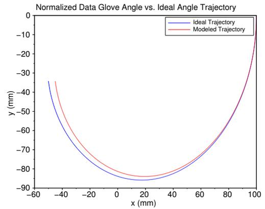
Figure 9: Normalized Data Glove Angle vs. Ideal Angle Trajectory
