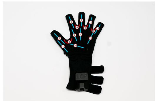
Figure 3: Fiber Sensor Placement of TELESAR V Data Glove after New Sensor Addition
