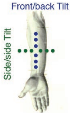
Figure 1: vibrating motor array layout
