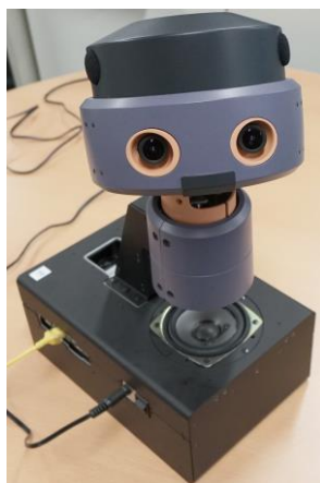
Figure 2. “TX-toolkit”, developed by JST-ACCEL Embodied Media Project, is a 3DOF robot-head equipped with communication functions for the experimental platform of teleexistence study.
