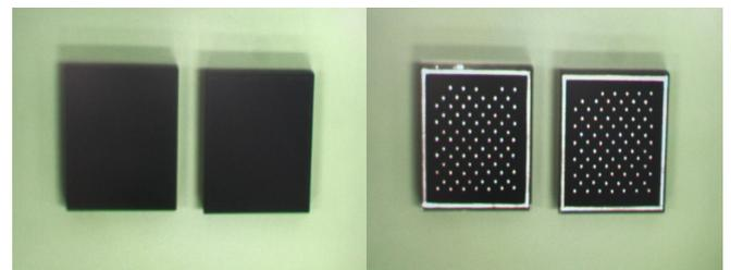
**Figure 6:** (left) Camera image without IR light. (right) Camera image under IR light. The inside of the interface is invisible to the naked eye. However, the use of the camera and IR light enables us to capture the view inside the interface. Each interface has different dot patterns, which enables ID detection.
