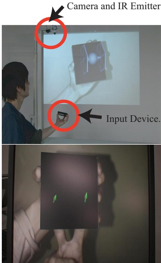
**Figure 4:** (Top) Appearance of proposed system. (Bottom) Captured image and force vectors. The green arrows show the force vectors applied by the user.
