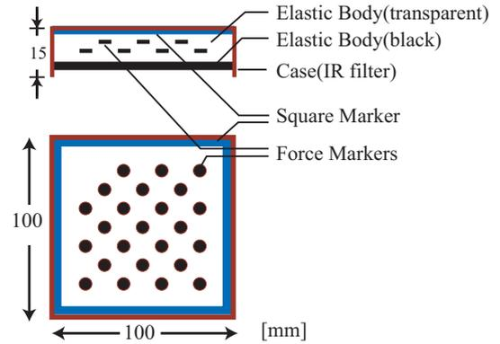
**Figure 5:** Structure of proposed interface.
