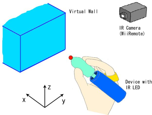
Fig. 7. Configuration of hardness detection experiment
