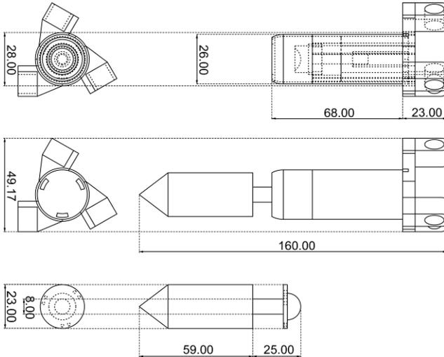
Fig. 4. Dimensional drawing of prototype device.
