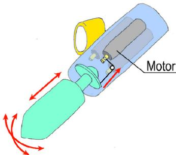
Fig. 2. Schematic of the mechanism of our proposed device
