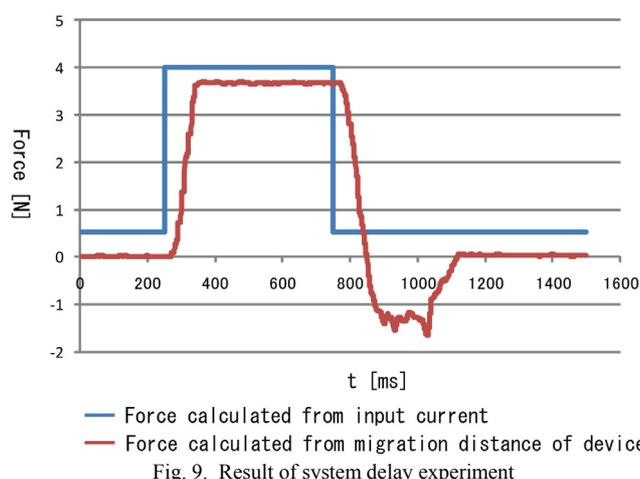
Fig. 9. Result of system delay experiment
