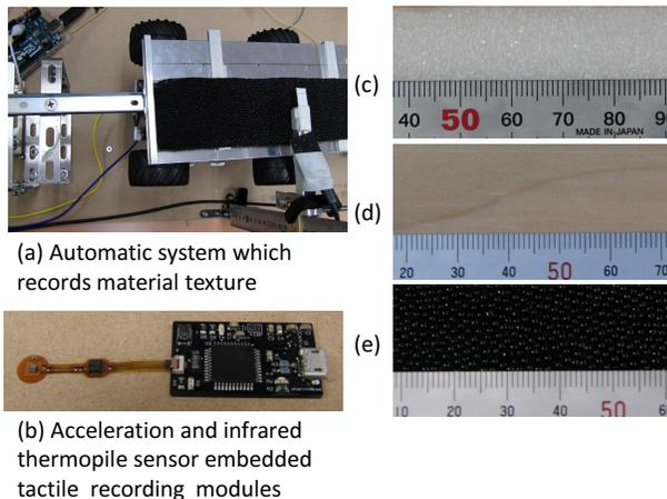
Figure 1: (a)Automatic system which records material texture, (b)Acceleration and infrared thermopile sensor embedded tactile recording module, (c) Urethane foam, (d) Board of Japanese Judas wood, (e) Ray skin plate.
