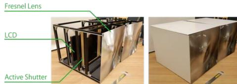
**Fig. 3.** Developed module overview
