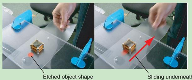
Fig. 5 Driving a pin-matrix by moving a texture
