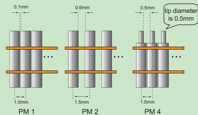
Fig. 7 Additional experiment for evaluating the space between the pin-rods
