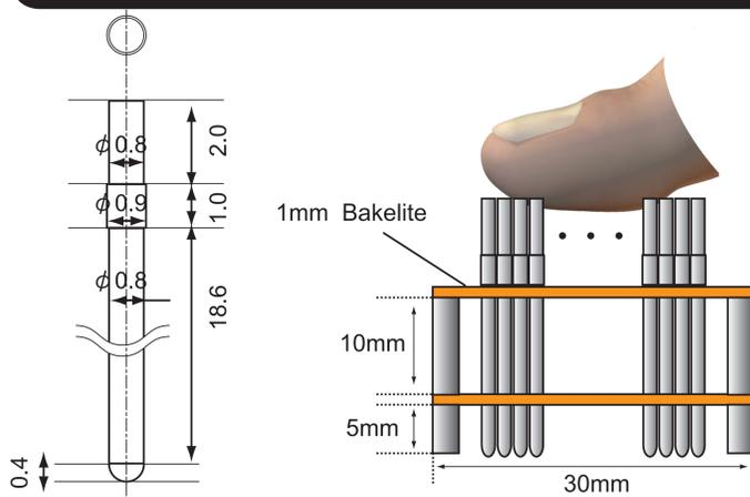
Fig. 1 Dimensions of the pin-rod
