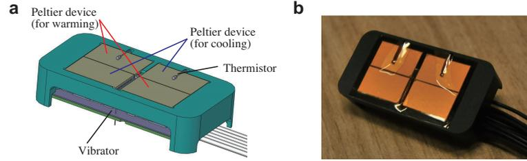
**Fig. 1.** Schematics (a) and developed (b) vibro-thermal tactile display
