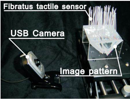
**Figure 8:** Overview of the sensor: The optic axis of the camera is located perpendicular to the captured surface
