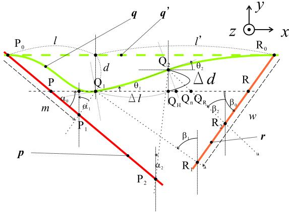
**Figure 5:** Geometrical optics: We express  $\Delta d$  with known values via  $\Delta\alpha$
