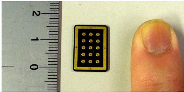
**Figure 2. Electrotactile display (Electrodes)**
