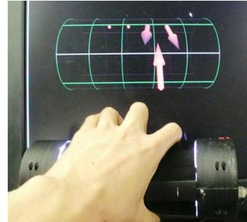
Fig. 5. Measured grip force. Green lines and red arrows represent the cylindrical shape of the device and the grip forces, respectively.
