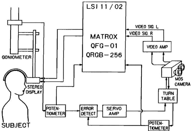
Figure 4 Schematic diagram of the experimental system
