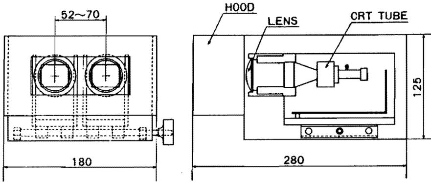
Figure 6 Binocular visual-display apparatus
