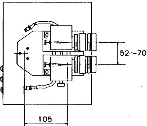
Figure 5 MOS TV cameras mounted on a turntable
