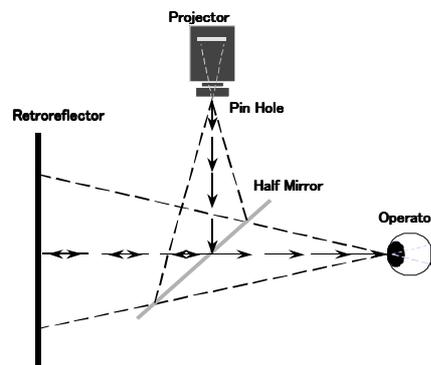
Fig.8 The Principle of RPT system.
