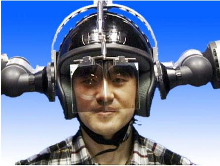
Fig. 12 General view of a Head Mounted Projector (HMP).
