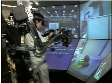
Fig.6 Telexistence Cockpit for Humanoid Control (2000).
