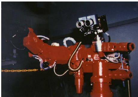
Fig. 2 Telexistence Surrogate Anthropomorphic Robot (TELESAR) at Work (1988).
