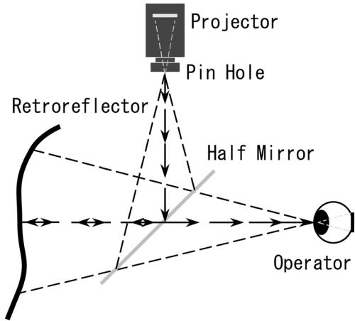
Fig.8 The principle of RPT system.
