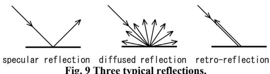
Fig.9 Three typical reflections.
