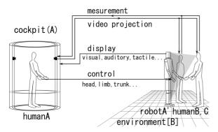
Fig.24 Schematic diagram of TWISTER used as a cockpit for robotic mutual t elexistence.
