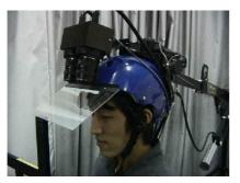
Fig. 11 General View of Head-Mounted Projector (HMP) used in this configuration.
