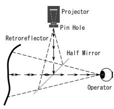
Fig.14 The principle of RPT system.
