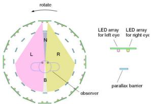
Fig.20 Principle of autosteropsis using moving parallax barrier.
