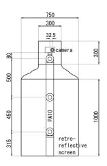
Fig.12 Configuration of Retro-reflective Screen Robot.
