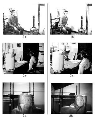
Fig. 13 Experimental Results: (1a, 1b) Human User A at Local Cockpit(A), (2a, 2b) Human User B and Telexistece Robot A' in Environment[B], and (3a, 3b) the image of the human user A on the robot A'. A black dot is where the camera is located.
