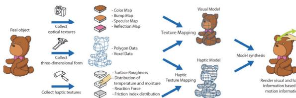
Figure 4: Technologies for Creation of Embodied Haptic Information Contents
