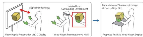
Figure 5: From Conventional 3D Visual-Haptic Displays to a 3D Visual-Haptic Display that Presents Reality
