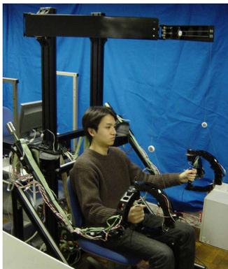
**Fig. 2** The whole view of the master arm
