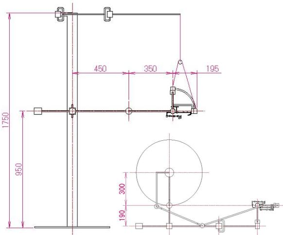
**Fig. 1** The whole schematic of the master arm
