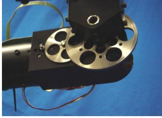
**Fig. 4** The gear system of the joint of the master arm
