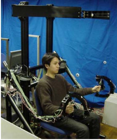
Fig. 3: The master arm of Telesar II
