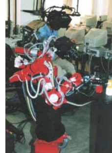
Fig. 1: The first telexistence master-slave system “Telesar I”
