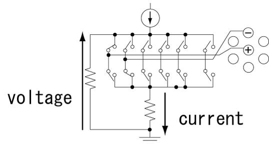
Fig. 4 Side paths to measure the voltage and the current
