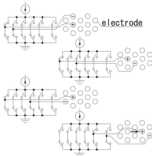
Fig. 1 Basic concept of the electro-tactile display with high-speed switching
