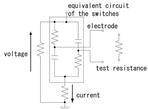
Fig. 15 Equivalent circuit of the switches
