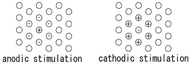
Fig. 7 Anodic and cathodic stimulation
