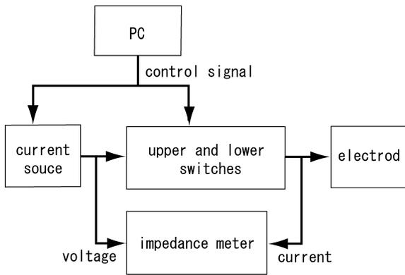
Fig. 8 Block diagram of the system
