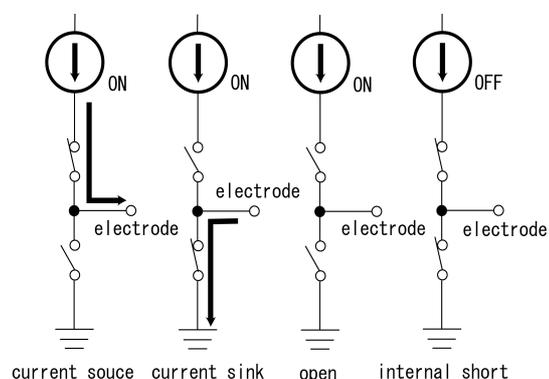
Fig. 2 Four states of electrode
