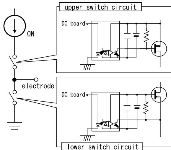
Fig. 10 Upper and lower switch circuit
