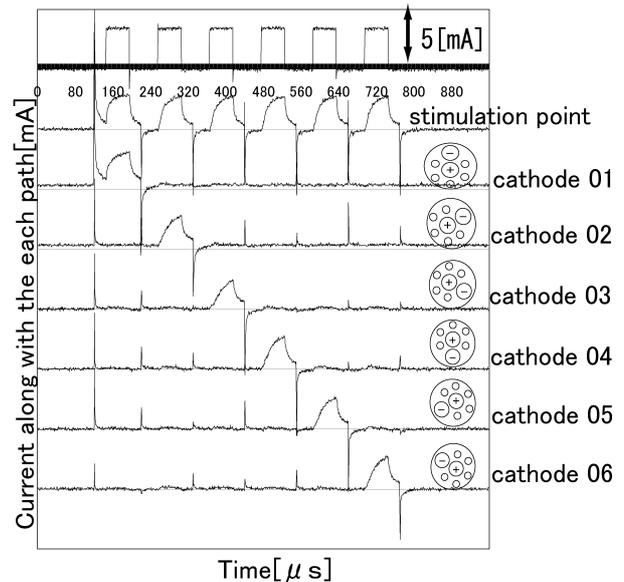
Fig. 14 Actual current through the electrodes
