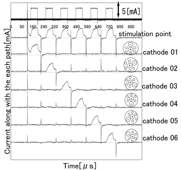
Fig. 14 Actual current through the electrodes
