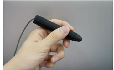
Figure 7. Prototype of the pen-shaped tactile device
