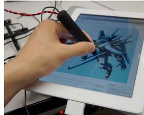
Figure 6. Using the pen-shaped tactile device
