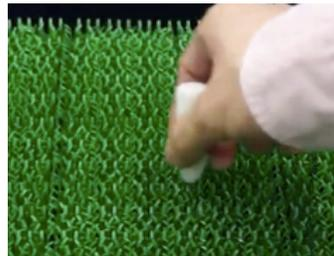
Figure 3. Recording tactile texture by using a microphone
