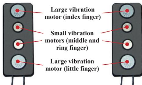
Fig. 10 HaptiTickler device.
