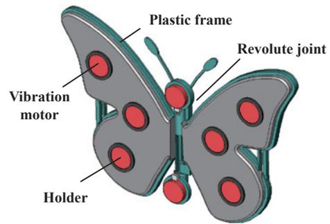
Fig. 8 Structure of HaptiButterfly.
