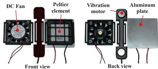
Fig. 9 Structure of HaptiShiver/HaptiTemper.
