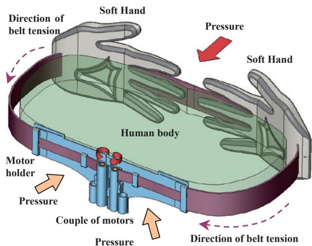
Fig. 6 Structure of wearable HaptiHug device.
