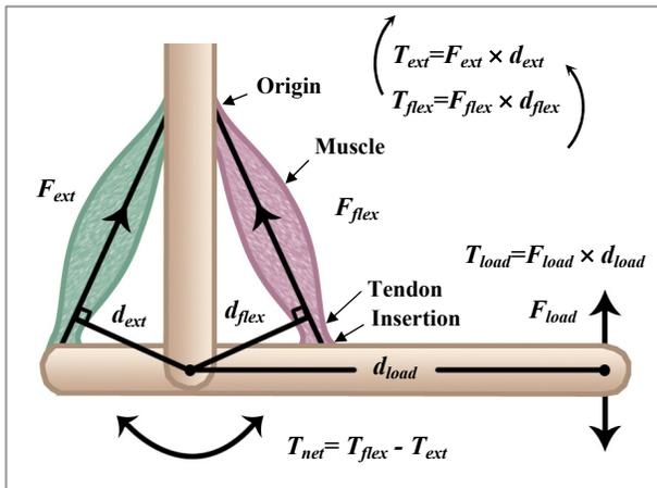
Figure 1. Structure and action of a skeletal muscle.
