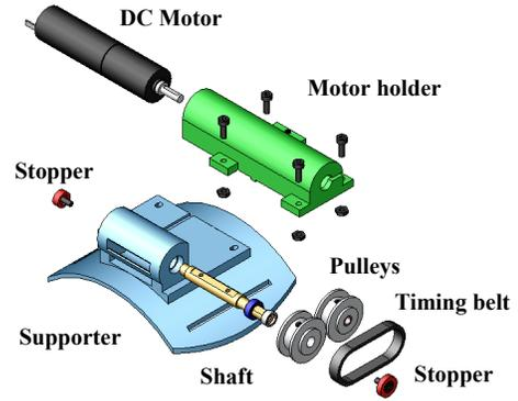
Figure 5. 3D exploded view of the driving unit of FlexTorque.
