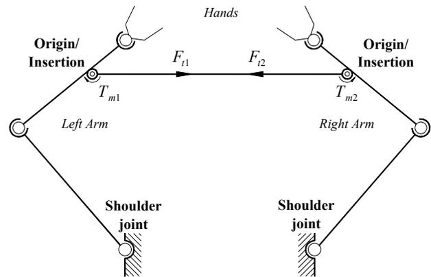
Figure 12. Kinematic diagram of FlexTensor and human arm.
