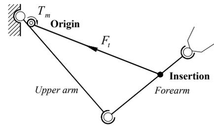
Figure 11. Kinematic diagram of FlexTorque and human arm.
