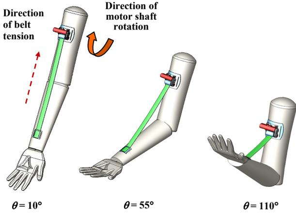
Figure 3. Positions of the human's arm under flexor torque.
