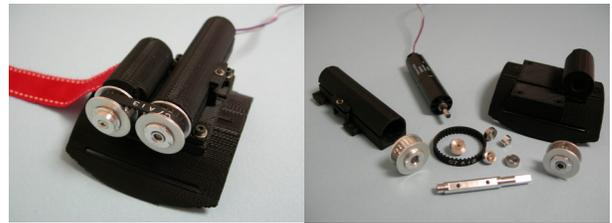
Figure 6. Driving unit of FlexTorque.
