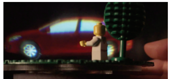
Fig5. Interaction with physical objects Rotating the 3D image by rotating the physical stage.
