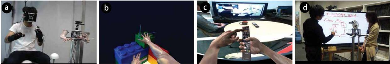
**Figure 1:** (a) *Superimposed Virtual Arms Concept on a Remote Telexistence Robot*, (b) *Touch and Feel Remote Objects using virtual arms*, (c) *Grabbing a Functional Virtual Copy of TV Remote*, (d) *Local-Remote Collaborative Digital Whiteboard*.
