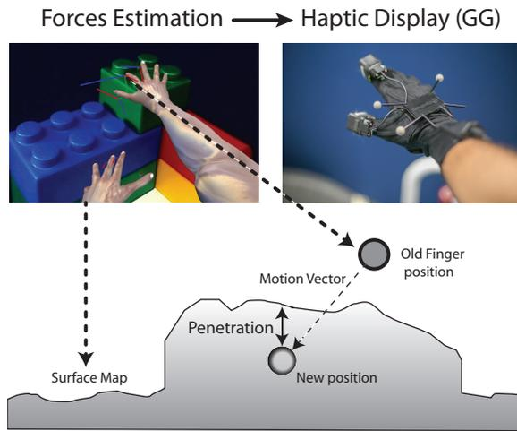
**Figure 3:** Calculating touch forces using the reconstructed 3D map and user fingers motion vectors, and applying the forces to the haptic display (GG)
