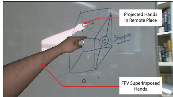
Figure 3. Superimposed hands on user's FPV, and the projected hands on robot's remote place.
