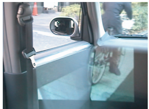
Figure 2: Implementation of the Transparent Cockpit. The lower part of a person riding a bicycle can be seen through the interior appointments of the car.
