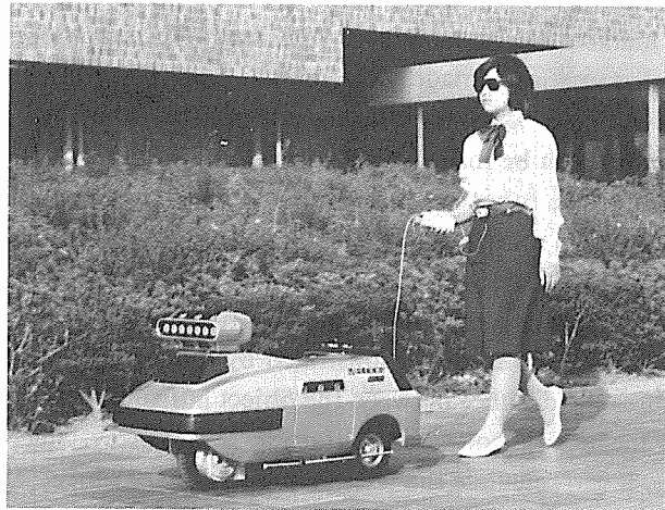
Fig. 2.5.9 General view of the guide dog robot MELDOG MARK IV. (Courtesy of the Mechanical Engineering Laboratory)
