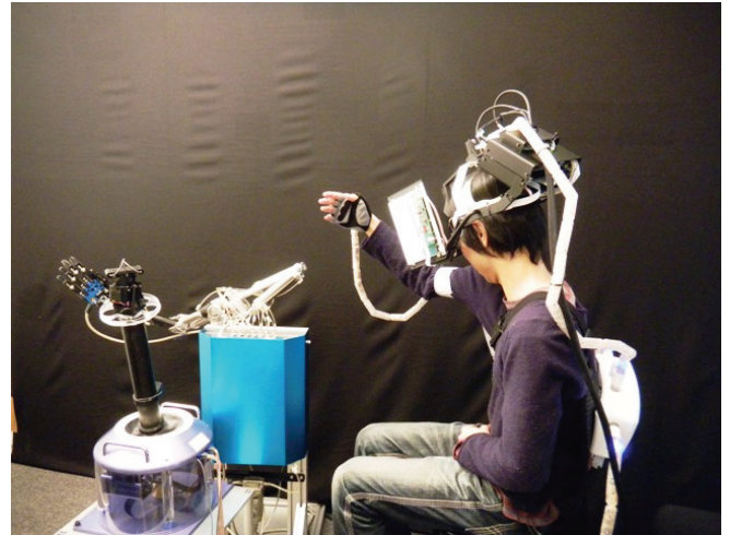
Fig. 2 : Overview of TELESAR3. (left: slave robot, right: operator and master)
