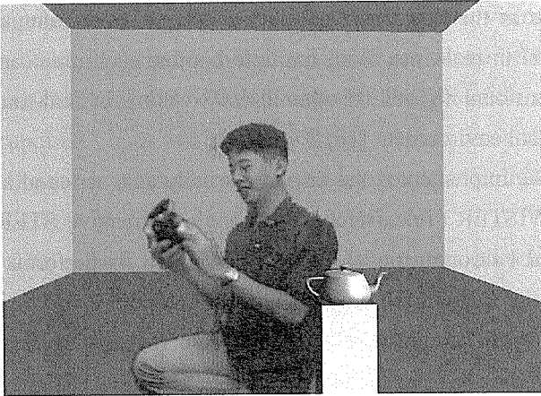
Figure 11: Constructed Human Figure. Images from an arbitrary viewpoint are constructed using rays captured by a camera array and placed in a virtual environment (adopted from [20]).
