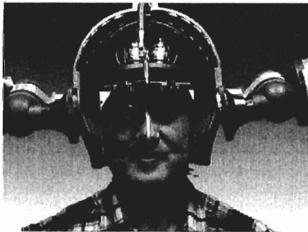
Figure 13: General view of a Head Mounted Projector (HMP).
