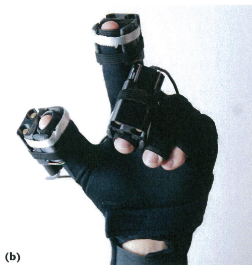
Figure 8. TELESAR V master and slave hands. (a) Slave hand with haptic sensors and (b) master hand with haptic displays.
