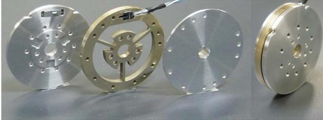
**Fig. 10.** Optical torque sensor with hub-spoke-shaped flexure.
