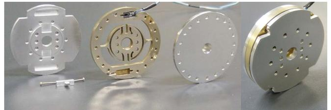
Fig. 18. Optical torque sensor with semi-ring-shaped flexure.
